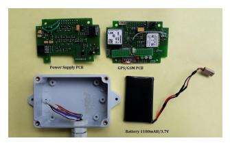
The tracker consists of a power supply PCB, GPS/GSM PCB and internal Battery.
