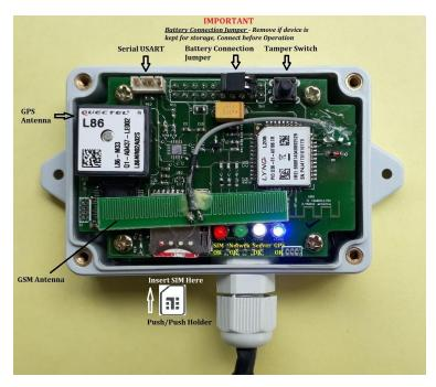
It is recommended that you connect the jumper only before closing the lid and ready to fit the device after inserting the SIM Card. The SIM Card holder is easily accessible (push push type connector). Please check the direction of insertion and the CUT on the SIM card. It is recommended that you turn off both external power as well remove the internal -Battery Connection Jumper- while changing the SIM card.
