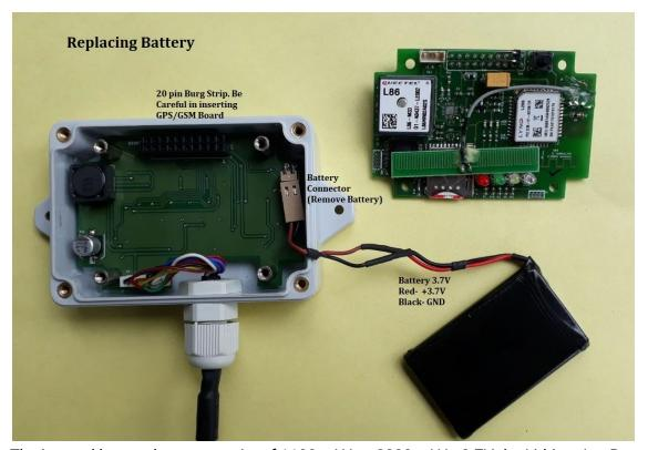
The internal battery has a capacity of 1100mAH or 2200mAH - 3.7Volts Lithium Ion Battery. The Battery can be changed by removing the GPS/GSM board.
